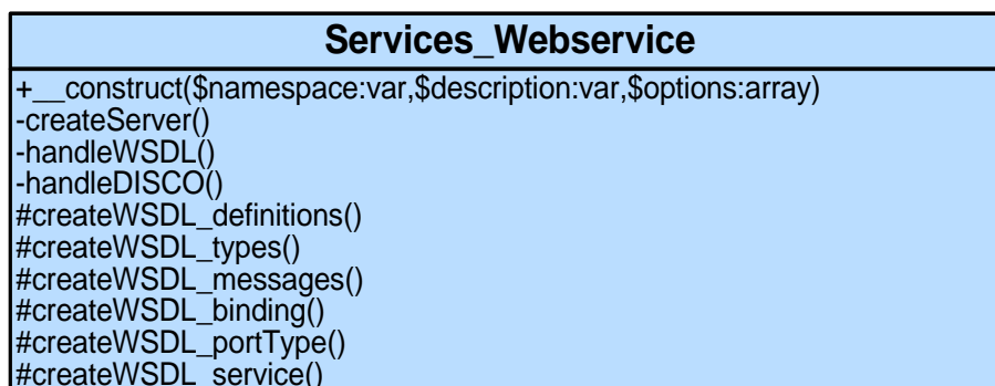
Figure 2.1.: UML Class Diagram of Services_Webservice . The Class attributes and some methods were omitted to make the Class more clear.
